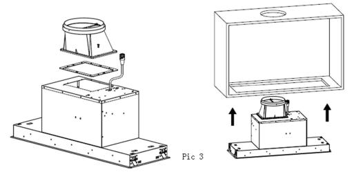
4. Put the hood into the cabinet, tighten up the screws by screwdriver, and make sure the hood was fixed. See Pic 4.
