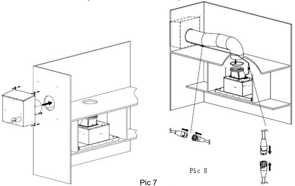
8. Install the expansion pipe onto the main body outlet and fix it with cable tie. Connect the motor extension wire both end with the external cabinet control wire and main body top control wire. The plastic base of the control wire should be plugged to the bottom, and make the bucket to tight status. See pic 8.
