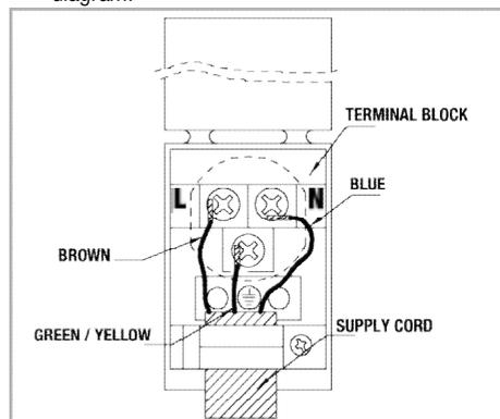
5. After completing the wire connections, close the terminal block cover.
