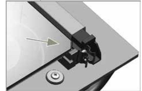
Inner glass panel (2) must be installed into the plastic slot close the innermost glass panel (1).
