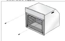
Secure the oven with 2 screws as illustrated. After the installation, make sure that the screws are sufficiently tightened and the oven does not move. Oven may tip over during use if it is not installed as per the instructions and if the screws are not sufficiently tightened.
