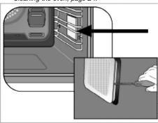
3. Remove the protective glass cover with a screwdriver.
