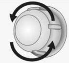
If your oven lamp is of type (A) shown in the figure below, remove it by rotating as shown and replace it. If it is of type (B), pull and remove it as shown in the figure and replace it.
