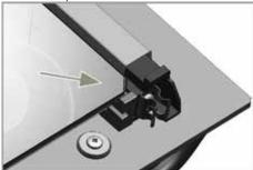
Inner glass panel (2) must be installed into the plastic slot close the innermost glass panel (1).
