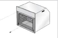
Secure the oven with 2 screws as illustrated. After the installation, make sure that the screws are sufficiently tightened and the oven does not move. Oven may tip over during use if it is not installed as per the instructions and if the screws are not sufficiently tiahtened.
