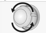
If your oven lamp is of type (A) shown in the figure below, remove it by rotating as shown and replace it. If it is of type (B), pull and remove it as shown in the figure and replace it.
