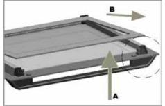
The first step to regroup the door is reinstalling inner glass panel (2).
