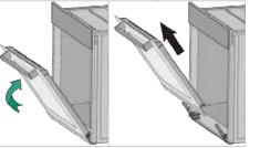
Remove the front door by pulling it upwards to 4. release it from the right and left hinges.
