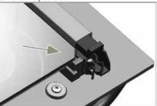
Inner glass panel (2) must be installed into the plastic slot close the innermost glass panel (1). When installing the innermost glass panel (1), make sure that the printed side of the panel faces towards the inner glass panel.
