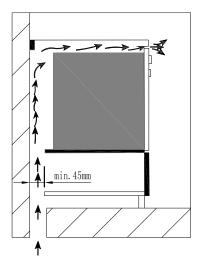
To provide adequate ventilation, there must be appropriate ventilation openings in the front bottom and the top part of 200 cm2, and an exhaust opening on the bottom of an least 200 cm2, and an exhaust opening of at least 60 cm2.
